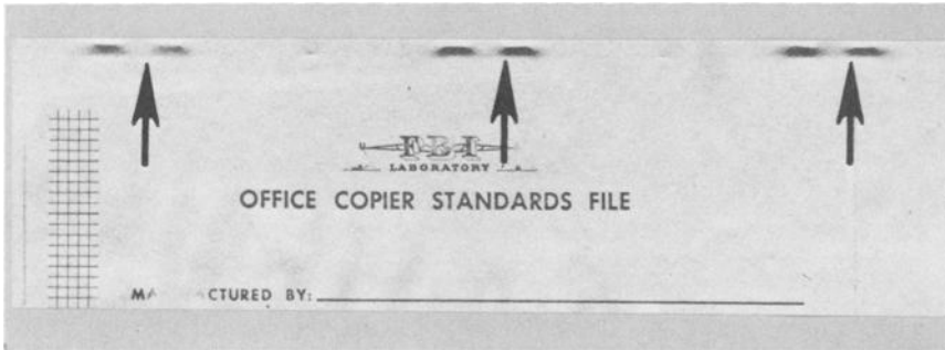
FIG. 5—Samples from Xerox 660 and 813 show gripper marks indented into top edge of the front side of the copy.
